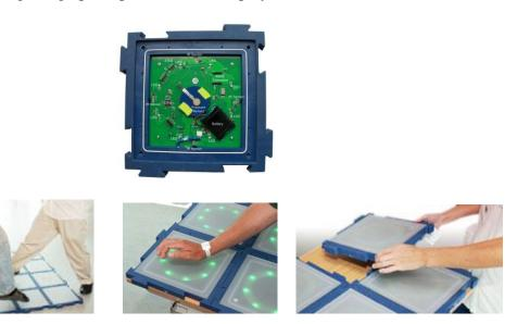
Figure 1: Modular tiles used for feet or hand interaction
